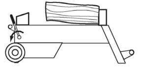
2. Insert a plastic or wooden Wedge under the jammed log (*Figure 12*) and activate the Ram to push the Wedge under the jammed log.
